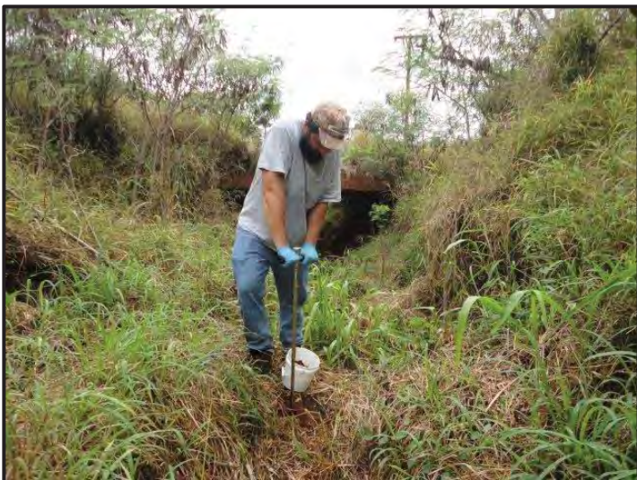
Photograph 3. A view of DU 2. Vegetation was cleared by DOW enough to access the drainage ditch. Entire continuous soil core plugs were collected using a hammer-head soil probe ( \frac{7}{8} -inch diameter). The soil plug was combined in a 2-gallon bag inside of a bucket to generate a bulk MI sample. Then, the MI sample was transferred into a plastic sealable bag, sealed, double-bagged, labeled, and placed in a chilled insulated chest (27 June 2018).
